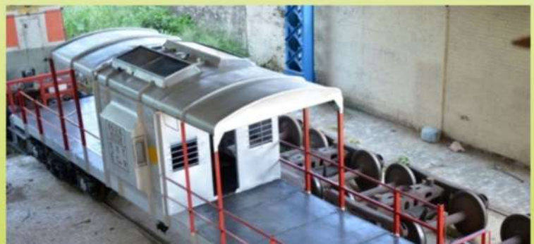
Renewable Solar Energy based Guard Comfort Kit in BVZi wagons
