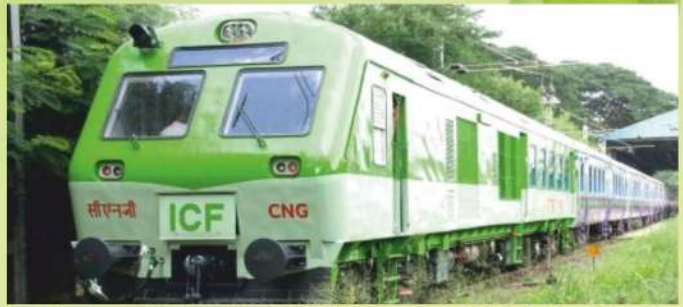
Environment friendly CNG in Dual Fuel Mode for Traction
